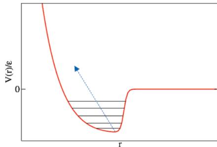
**Figure 1.** Schematic depiction of an isotropic pair interaction with a softened interior in its basin of attraction. Thermal fluctuations cause the average nearest-neighbor distance to decrease, resulting in an overall contraction of the system upon heating. Here, the horizontal black lines within the basin represent temperature values, and the broken line represents the thermally averaged nearest-neighbor distance.
