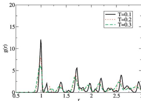
**Figure 13.** Radial distribution function for the SIC system in three dimensions at  $p = 1.0$  for three temperatures,  $T^* = 0.1, 0.2,$  and  $0.3$ . As a result of the increasing curvature of the SIC potential, given in eq 6, near its minimum, the first peak is increasingly skewed to smaller  $r$  as the temperature is increased. The second peak is not present in the perfect fcc lattice and represents a shearing of the system.
