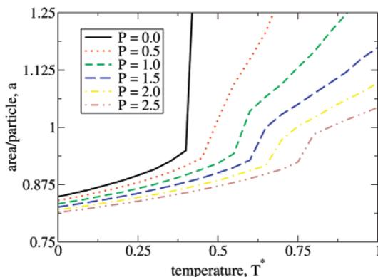
**Figure 8.** Specific area as a function of temperature for a number of different pressure values for the two-dimensional Lennard-Jones system. These results are obtained from NPT Monte Carlo simulations with  $N = 1040$  particles and periodic boundary conditions. In its crystalline (triangular) state, this system expands when temperature is increased for all pressures and temperatures. Note that kinks in the curves indicate melting of the crystal.
