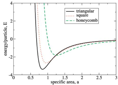
**Figure 4.** Two-dimensional lattice sums for the Lennard-Jones potential including the triangular, square, and honeycomb lattices. The lowest overall energy structure is the triangular lattice, which is thus the stable structure at zero pressure. From the Maxwell construction, we find that the pressure range of stability at zero temperature is  $0 < p < \infty$ , and the range of stability in specific area is  $0 < a < 0.85$ .
