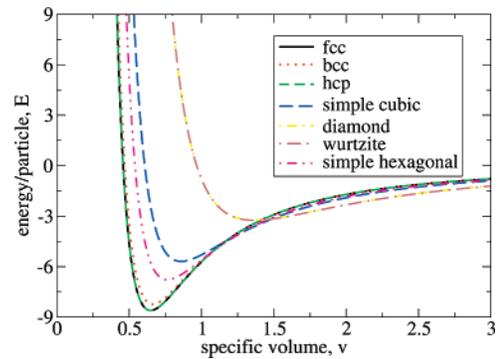
**Figure 5.** Three-dimensional lattice sums for the Lennard-Jones potential including the fcc, bcc, hcp, simple cubic, diamond, wurtzite, and simple hexagonal lattices. The lowest overall energy structure is the hcp lattice, which is thus the stable structure at zero pressure. From the Maxwell construction, we find that the pressure range of stability at zero temperature is  $0 < p < 1240$ , and the range of stability in specific area is  $0.33 < v < 0.65$ .
