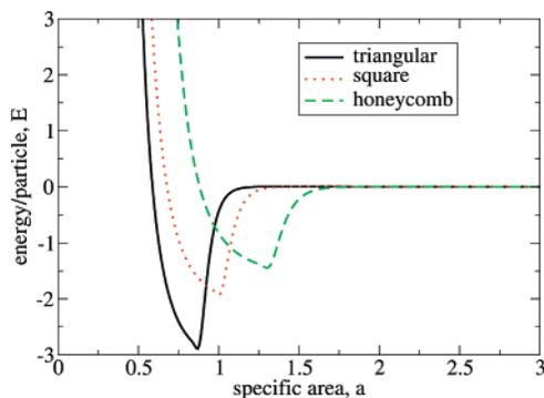
**Figure 6.** Two-dimensional lattice sums for the SIC potential including the triangular, square, and honeycomb lattices. The lowest overall energy structure is the triangular lattice, which is thus the stable structure at zero pressure. From the Maxwell construction, we find that the pressure range of stability at zero temperature is  $0 < p < \infty$ , and the range of stability in specific area is  $0 < a < 0.87$ .
