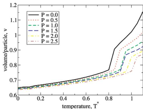
**Figure 9.** Specific volume as a function of temperature for a number of different pressure values for the three-dimensional Lennard-Jones system. These results are obtained from NPT Monte Carlo simulations with  $N = 864$  particles and periodic boundary conditions. In its crystalline (fcc) state, this system expands when temperature is increased for all pressures and temperatures. Note that the “kinks” in the curves indicate melting of the crystal.
