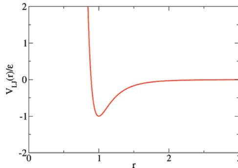
**Figure 2.** Lennard-Jones potential, as given in eq 3, with  $\epsilon_{LJ} = \epsilon$  and  $\sigma_{LJ} = 1/2^{1/6}$ . As can be easily seen, the curvature of the potential is greater to the left of the minimum at  $r = 1$  than to the right. As a result, when the temperature of a system interacting via this potential is increased, thermal fluctuations cause the average nearest-neighbor distance to increase.
