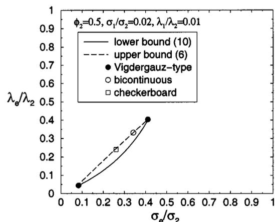
FIG. 10. Cross-property bounds and simulation data for the effective electrical  $\sigma_e$  and thermal  $\lambda_e$  conductivities for well-ordered phases ( $\sigma_1/\sigma_2 < 1$  and  $\lambda_1/\lambda_2 < 1$ ) as specified by Eq. (14).
