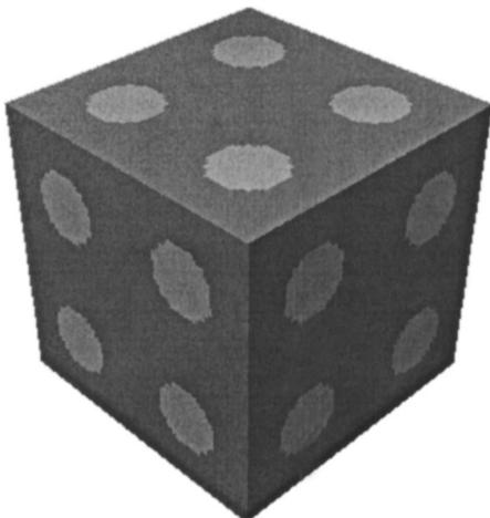
FIG. 3. A bicontinuous optimal structure at  $\phi_1 = \phi_2 = 1/2$  corresponding to maximization of the sum of the effective electrical and thermal conductivities ( $\sigma_e + \lambda_e$ ) for ill-ordered phases in which  $\sigma_1 = 0.1$ ,  $\sigma_2 = 1$ ,  $\lambda_1 = 1$ ,  $\lambda_2 = 0.1$ . Shown is a  $2 \times 2 \times 2$  unit cell.
