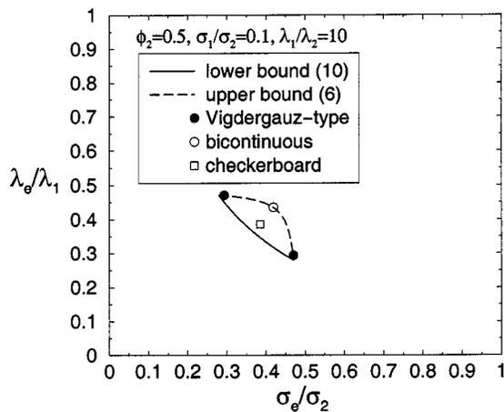
FIG. 8. Cross-property bounds and simulation data for the effective electrical  $\sigma_e$  and thermal  $\lambda_e$  conductivities for ill-ordered phases ( $\sigma_1/\sigma_2 < 1$  and  $\lambda_1/\lambda_2 > 1$ ) as specified by Eq. (13).
