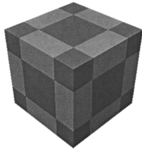
FIG. 9. At  $\phi_1 = \phi_2 = 1/2$ , the three-dimensional checkerboard is the best single-scale structure that we obtained when both properties are minimized with same weighting factors. Shown is a  $2 \times 2 \times 2$  unit cell. Note that this structure does not achieve the lower bound of the sum of the two conductivities obtained from the cross-property relation (7), as shown in Fig. 8.
