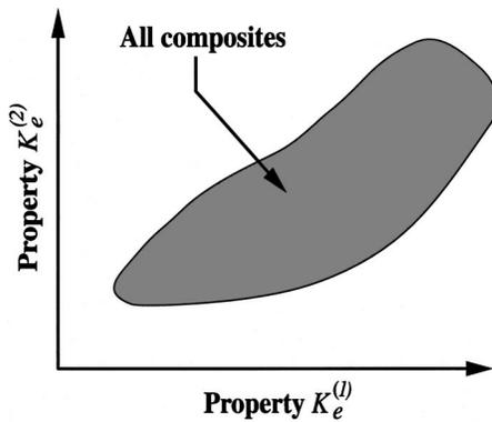
FIG. 1. Schematic illustrating the allowable region in which all composites with specified phase properties must lie for the case of two different effective properties.
