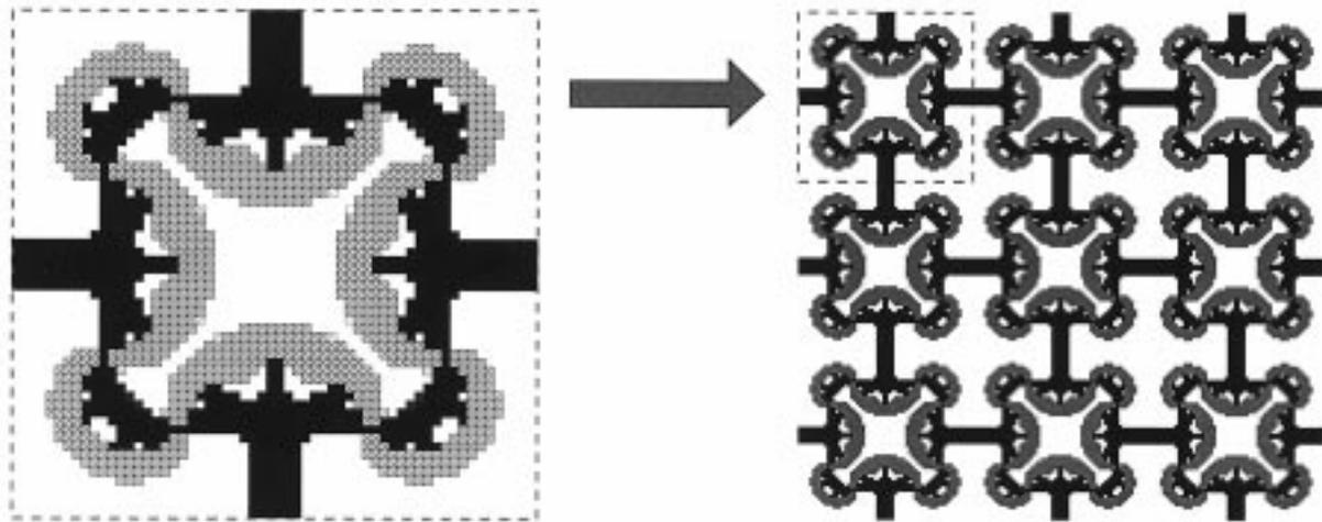
Fig. 4. Optimal microstructure for minimization of effective thermal expansion coefficient (Sigmund and Torquato, 1997). White regions denote void, black regions consist of low expansion material and cross-hatched regions consist of high expansion material.
