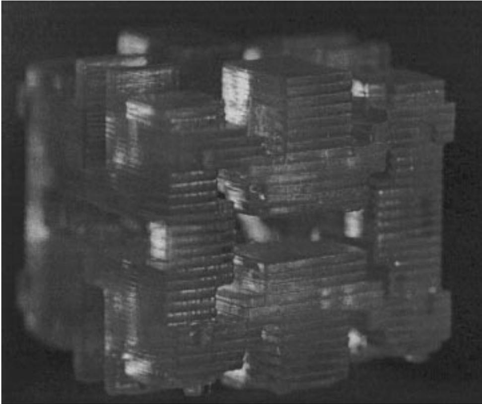
Fig. 5. Prototype of one base cell made by stereolithography. This special porous solid has negative Poisson's ratio and, when used as a matrix in a piezocomposite, maximizes hydrophone performance.
