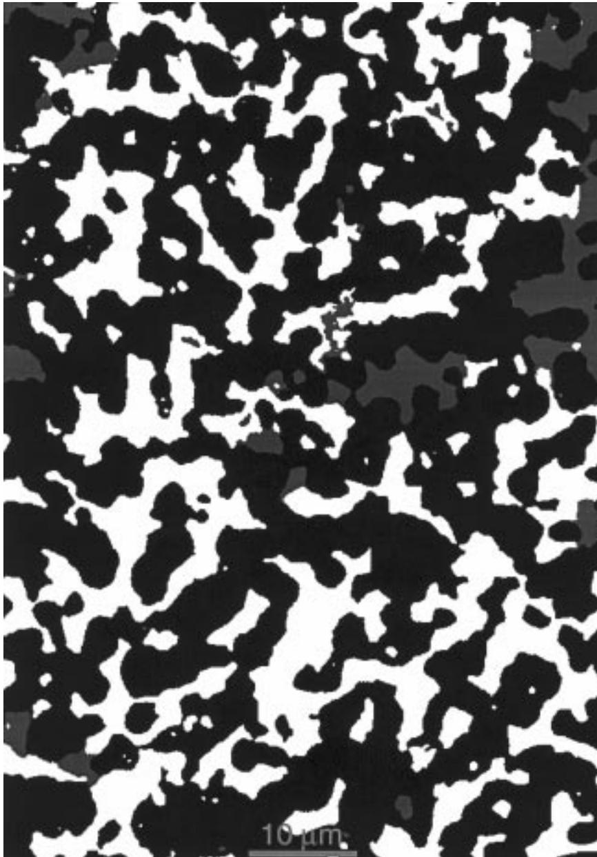
Fig. 1. Gray-scale digitized microscope image of a three-phase boron carbide/aluminum composite: white region is Al phase, black region is B<sub>4</sub>C phase, and gray region is Al<sub>4</sub>BC phase. The B<sub>4</sub>C and Al phases are the dominant ones.
