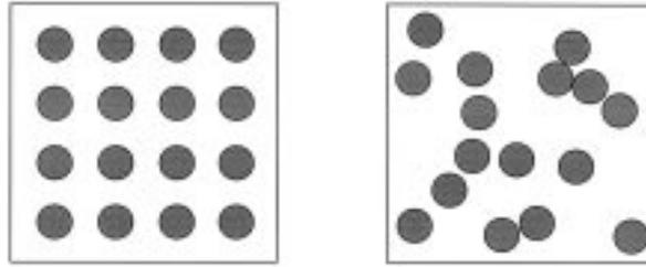
Fig. 2. Two systems at the same volume fraction but the right-most example has greater fluctuations. The failure characteristics of these systems can be dramatically different from one another.
