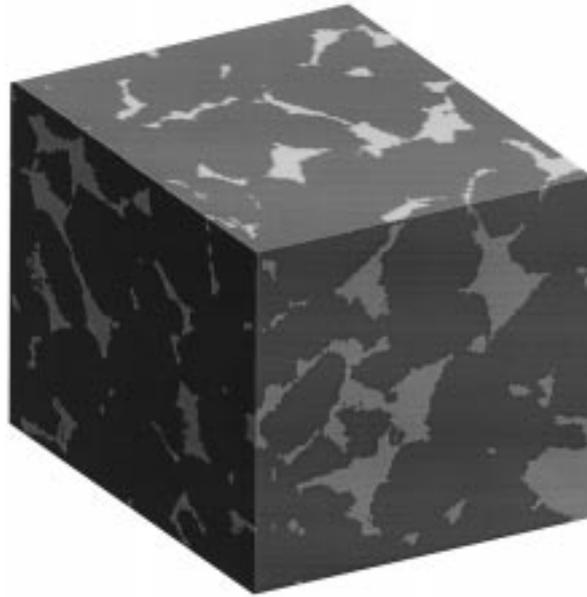
Fig. 3. Fontainebleau sandstone: lighter shade is void and darker shade is solid.
