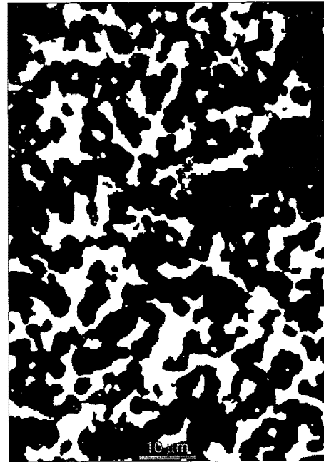
Fig. 6. Gray-scale digitized image of sample B (white region is Al phase, black region is B 4 C phase, and gray region is Al 4 BC phase). System size is 602 pixels \times 872 pixels.
